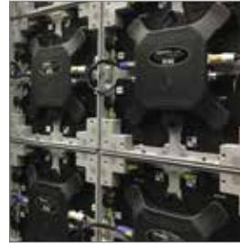
The tiles are aligned using magnets, whilst two manual connectors ensure a strong connection.
