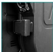
Toolless tighteners for quick and easy attachment of the power box
